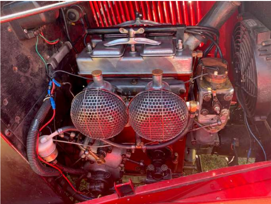
Sacha Leemann's '32 Nine tourer is still fitted with a fully functioning magneto.
