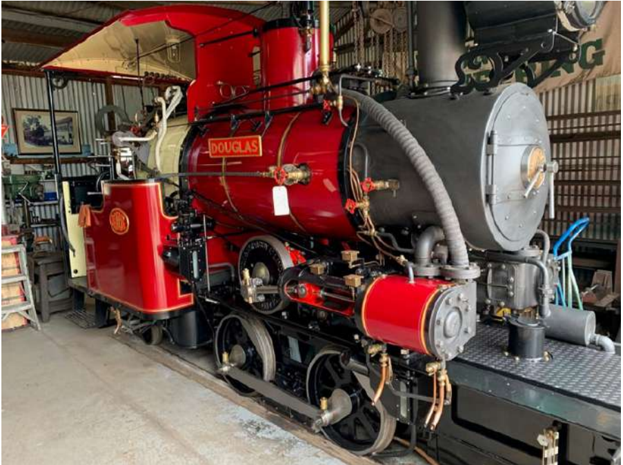
"Douglas" the wood fired gear driven steam locomotive built by Andrew Forbes.
