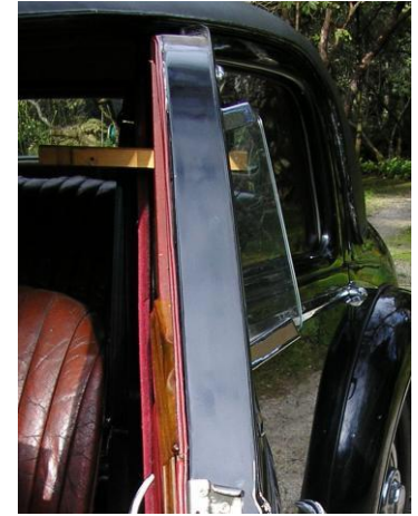
EARLY CAR. NO RUBBER DOOR SEAL
