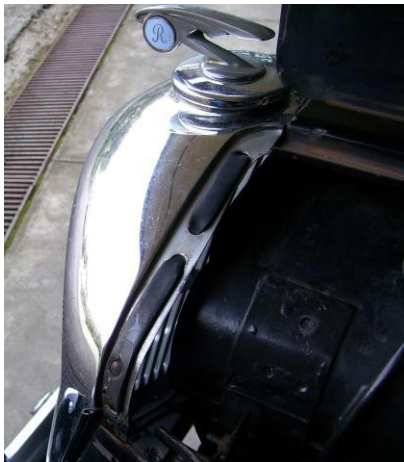
Bonnet closing strip on grill. Can be webbing or rubber.
