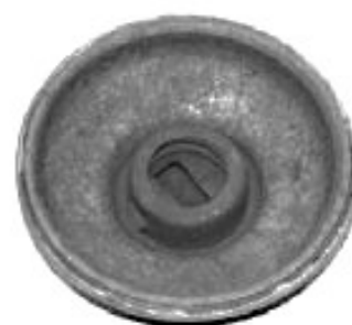
Underneath side of the lid with its spring mounted cam plate
