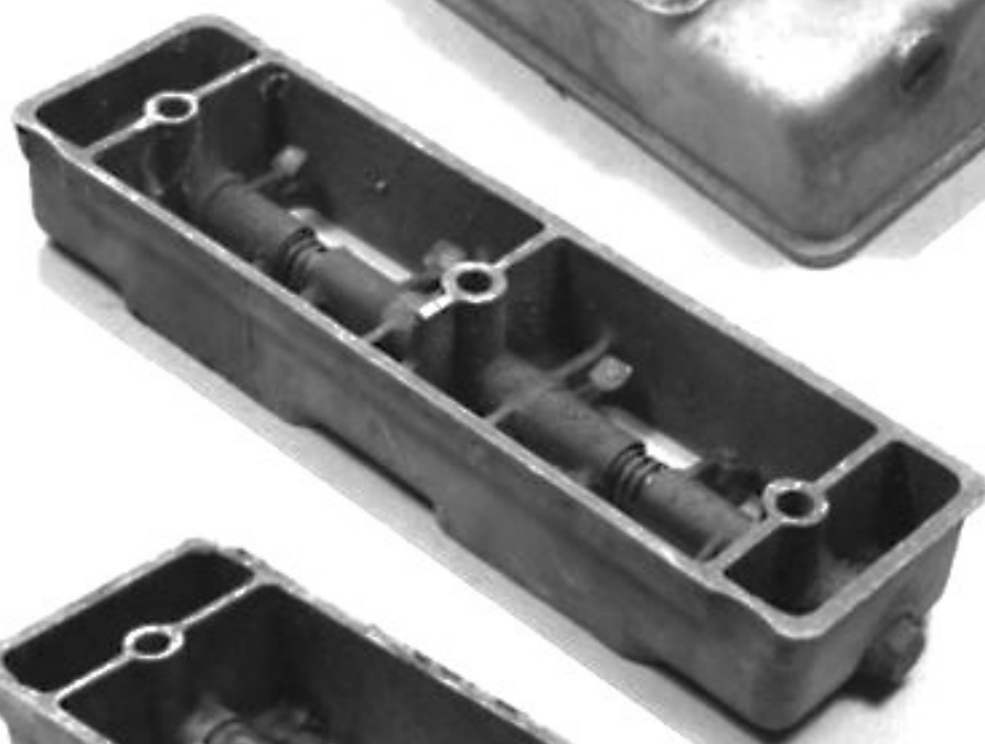
The Mk 2 up to Mk 5 engines had external piping for oil feed to the rocker shaft and this image shows an inlet side unit
